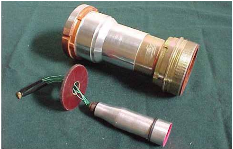
Throat-based igniter with nozzle
