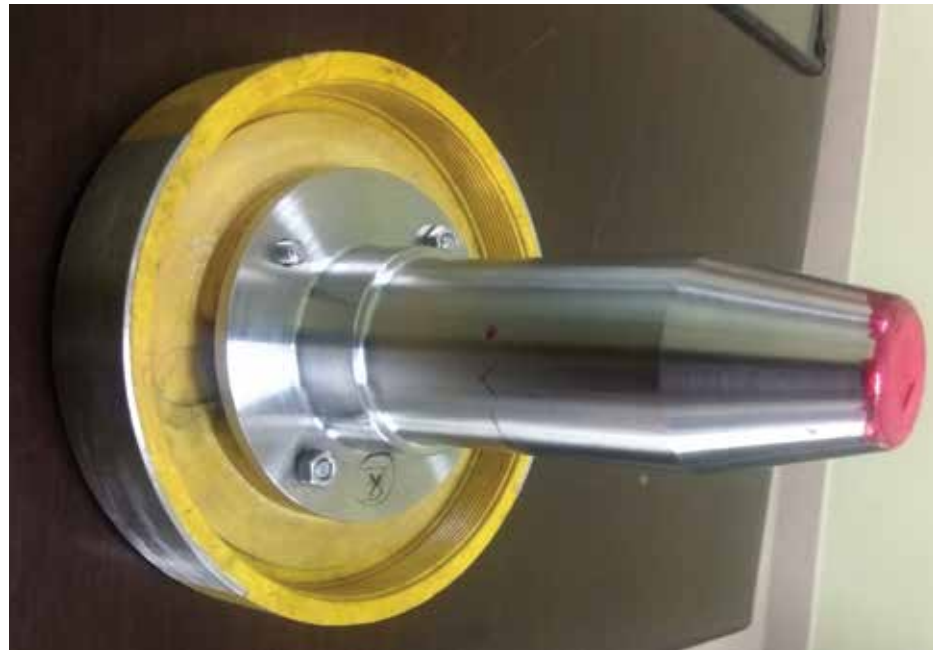
Cap-based ignition system assembly
