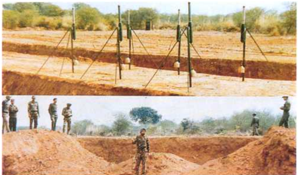
An array of six bund blasting devices at blast site (above). Crater formed after the blast (below)
