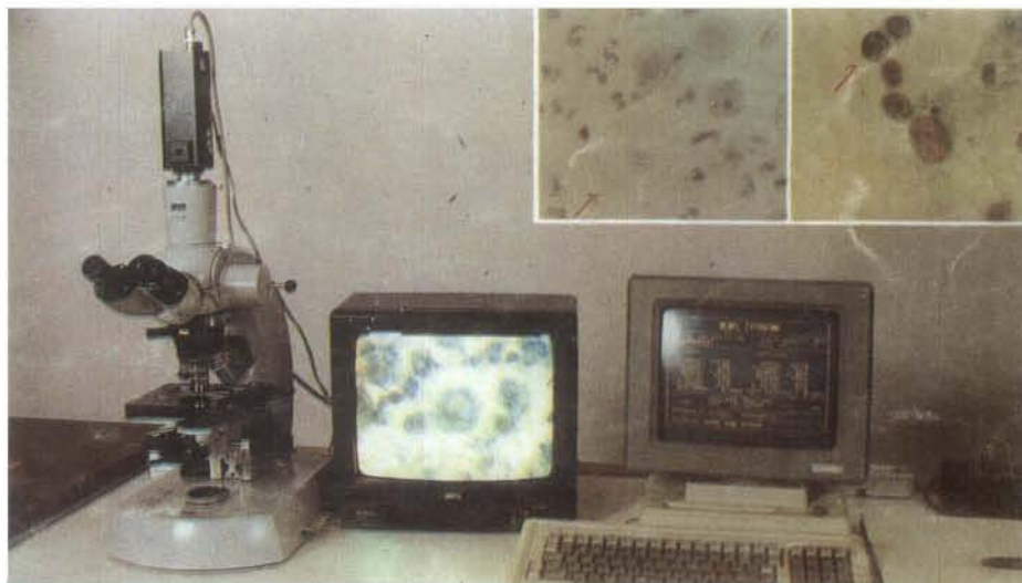
Cytoscan —a computer interactive system for cell morphometry. Inset: A view of parabasal (left) and cancerous (right) cells identified in Cytoscan
