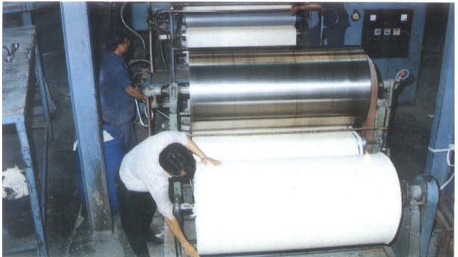
Coating of balloon fabric on zimmer coating machine at Entrmonde Polycoaters, Nasik
