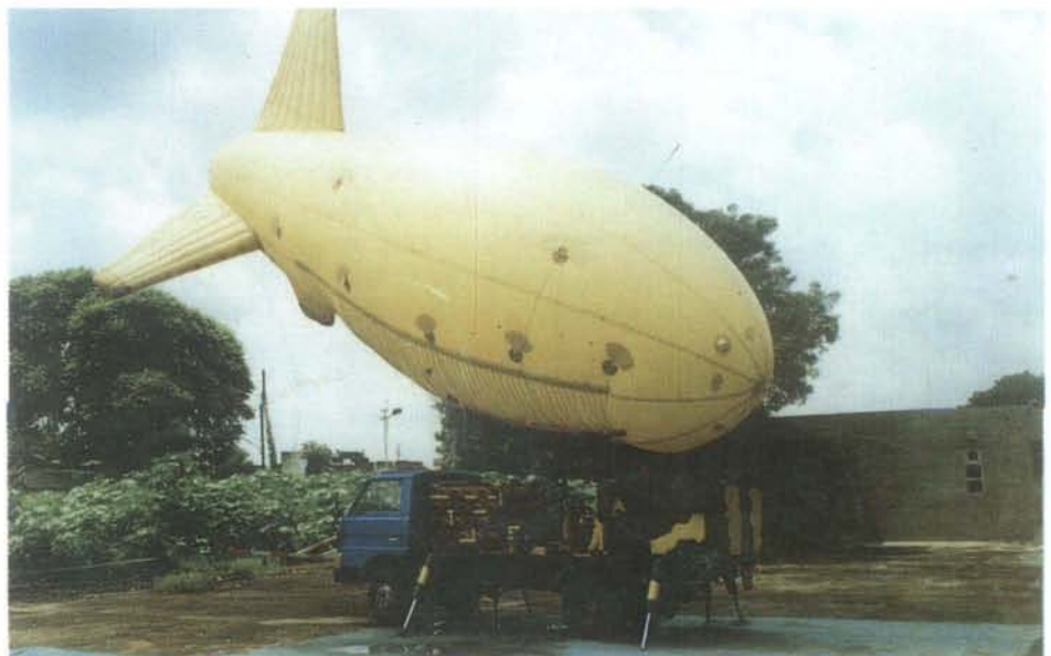
A unit of relocatable balloon barrage system
