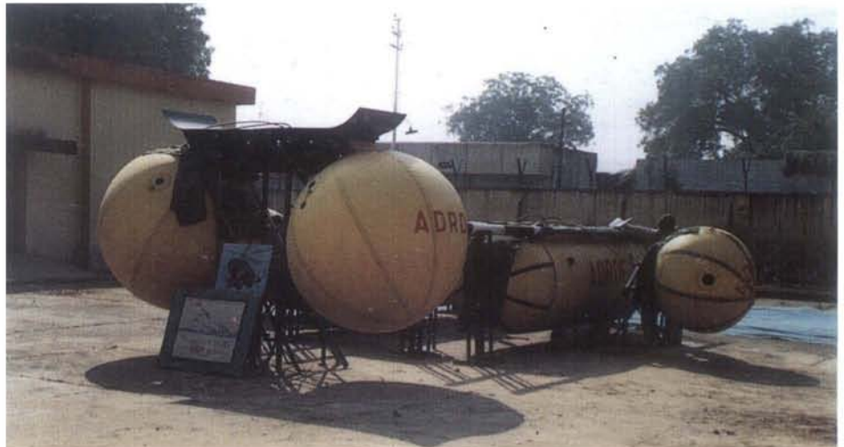
Ground testing of floats for emergency flotation system for MI-8 Helicopters on a mock-up
