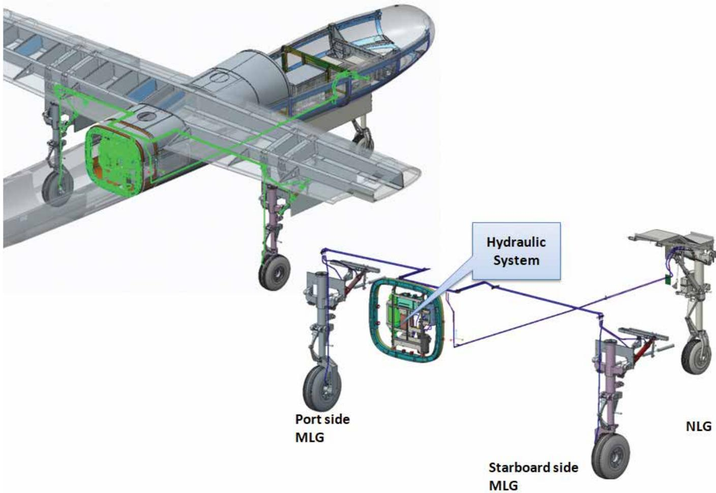
Schematic of RLG Hydraulics system of Tapas UAV
