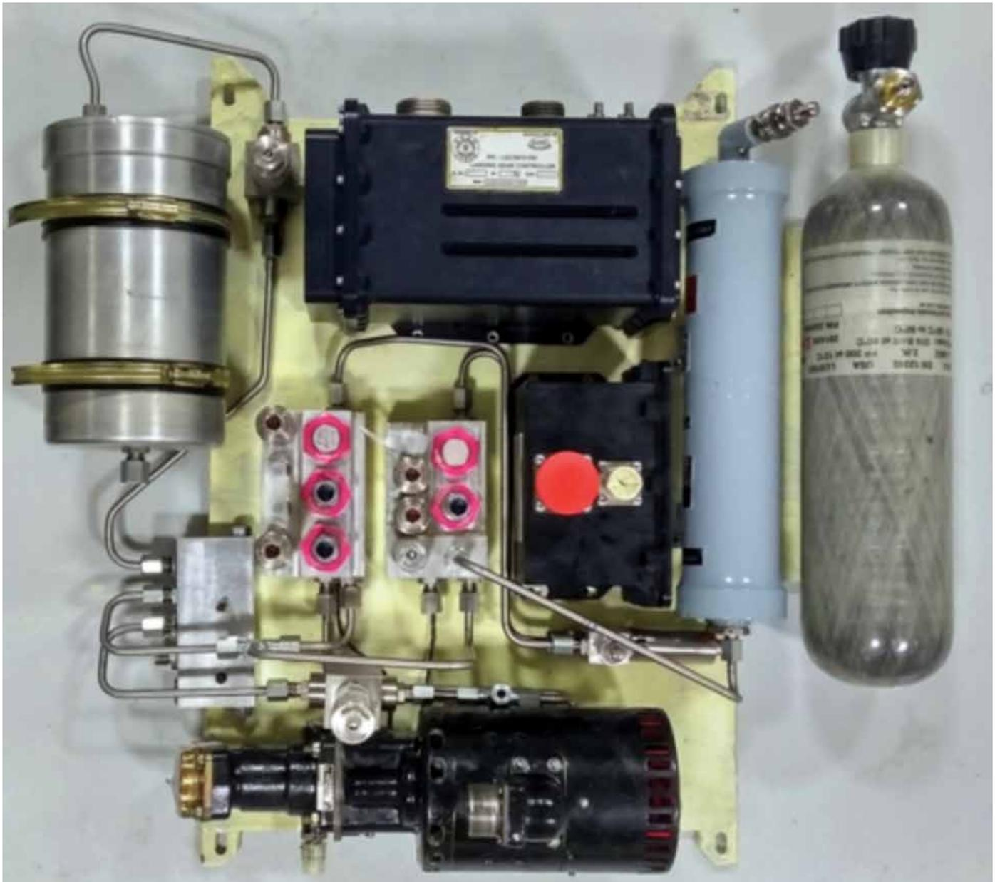
**RLG Hydraulics System of Tapas UAV**
