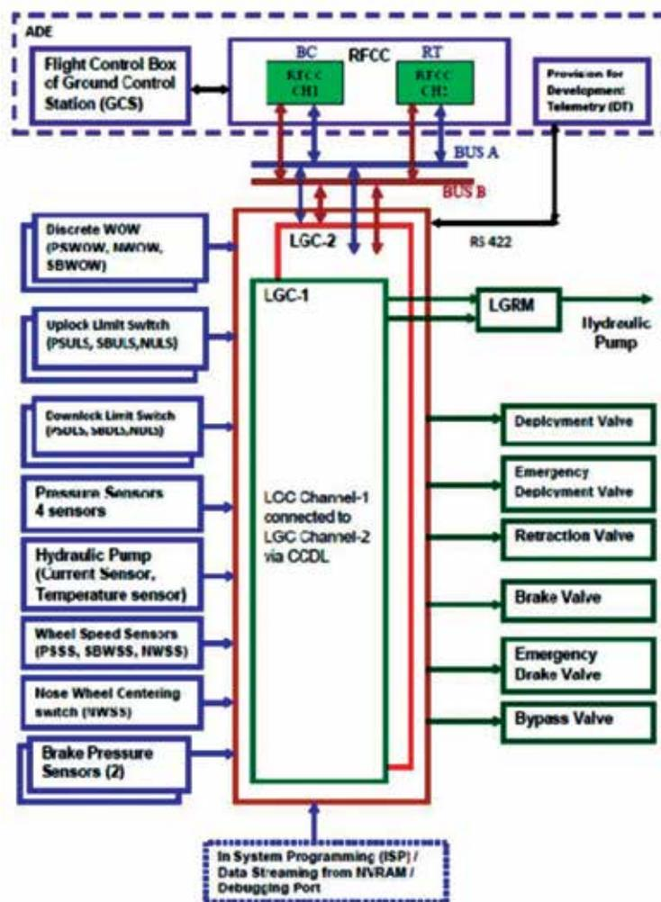
Block diagram of Landing Gear Controller
