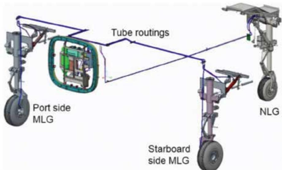
Landing gear system for Tapas UAV
