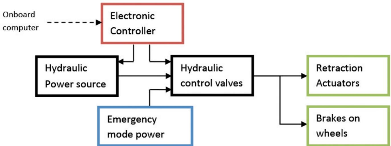
Block diagram of RLG Hydraulics system of TAPAS UAV
