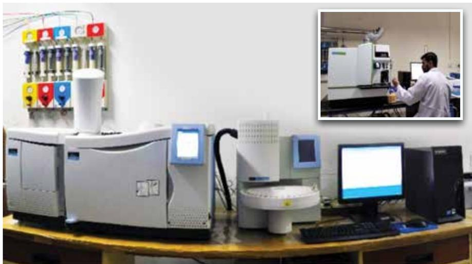
Gas chromatograph with Mass Spectrometer. Inset: Inductively Coupled Plasma Mass Spectrometer
