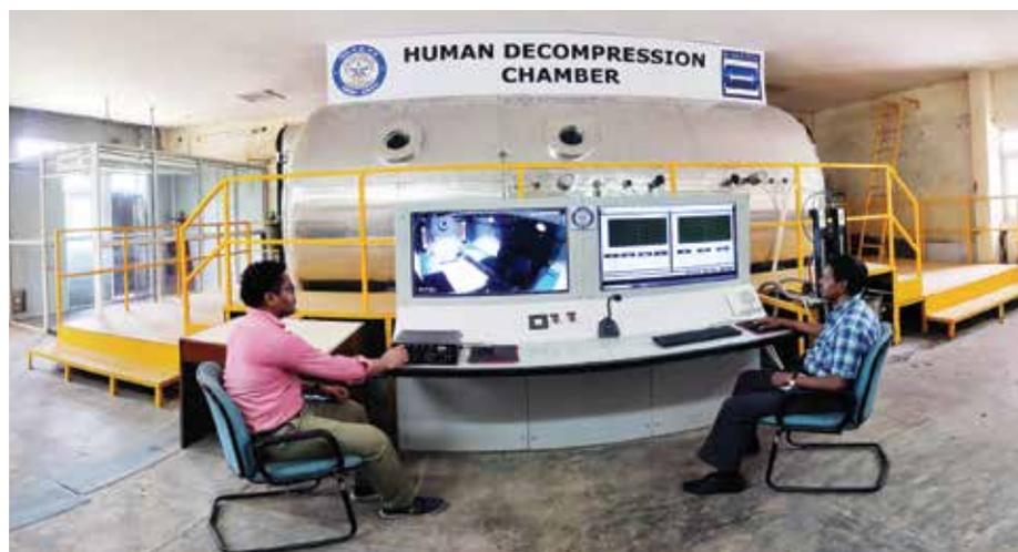
Human Decompression Chamber for Simulation of Cold and Altitude
