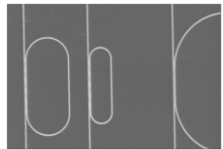
SEM image of a micro-ring resonator using photonic wire waveguides, fabricated by e-beam lithography
