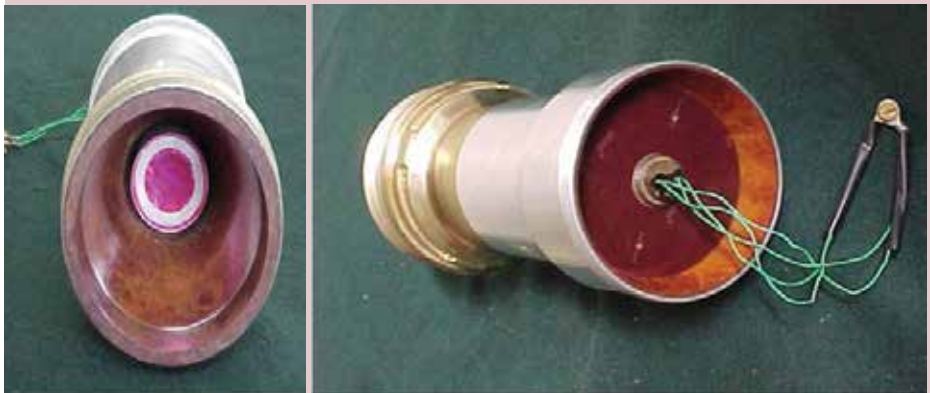
Throat based igniter fitted inside nozzle Throat View & Divergent view
