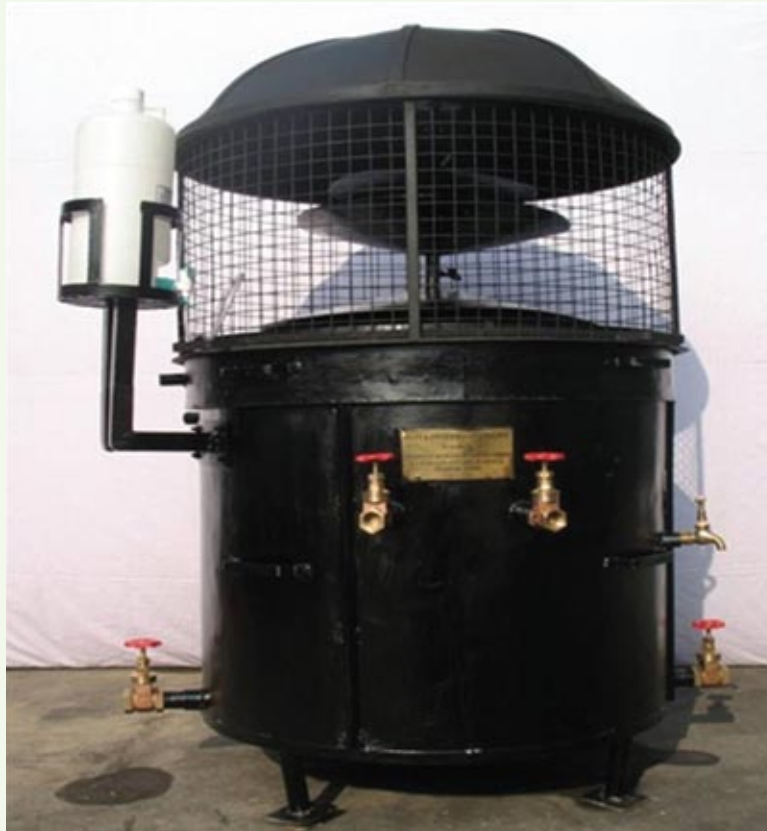
Water Dearsenification cum Deferrization Unit (200 L/h )
