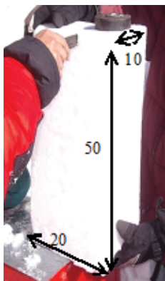
Determination of interfacial snow fracture energy release rate for interface involving FCso snow.
