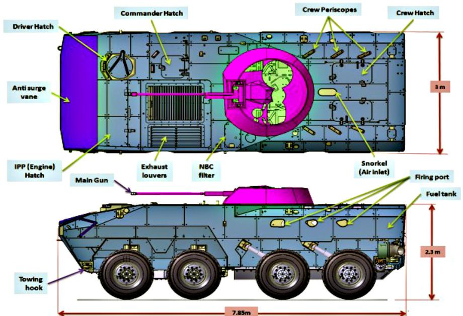
Wheeled Armoured Vehicle and its Structural Diagram (below)
