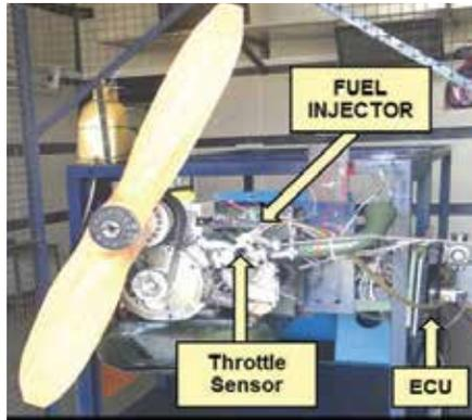
Rotary engine with EFI system on test bed
