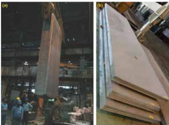
Indigenised AA2519 (a) Slab, and (b) T87 Plates (t = 15 mm) produced at BALCO
