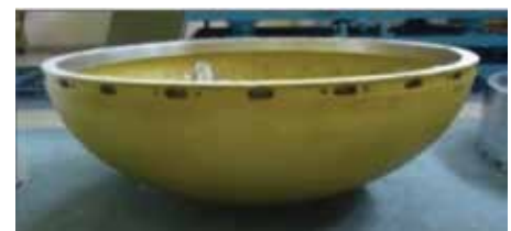
Nose cap dome, fabricated from indigenised AA2219-O plate
