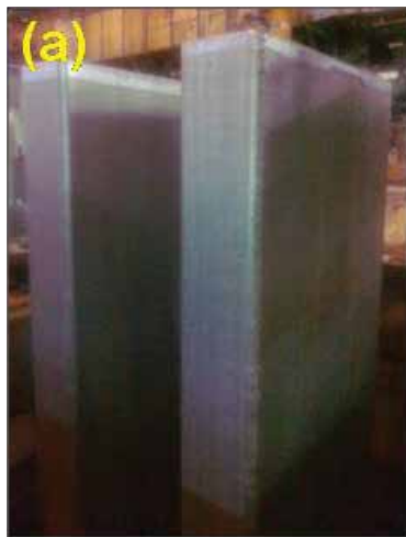
Indigenised Al-Mg alloy DMR291A in the form of (a) as-cast ingots, (b) M plate (t = 25 mm), and (c) H24 sheets (t=2 mm) produced at BALCO, Korba
