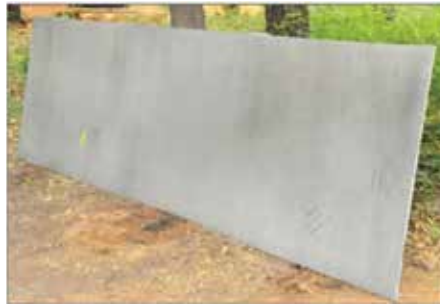
Indigenised AA2519-T87 plate (t = 10 mm) produced at BALCO, Korba
