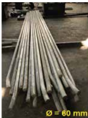
Indigenised AA6082-T651 extrusions produced at OFAJ, Nagpur
