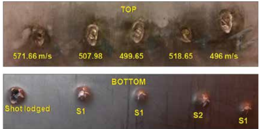
Top and bottom sides of the 15 mm thick AA2519-T87 plate subjected to the ballistic test against 7.62 x 54 mm AP (I) ammunition
