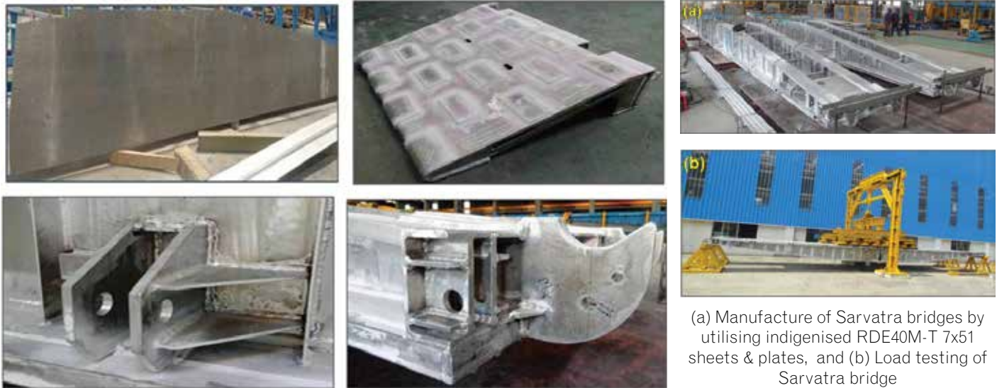
Different parts of the Sarvatra bridge such as (a) Web plate, (b) Ramp assembly, (c) Lifting hook, and (d) Pier bracket as fabricated from the indigenised RDE40M-T 7x51 sheets and plates having different thicknesses
