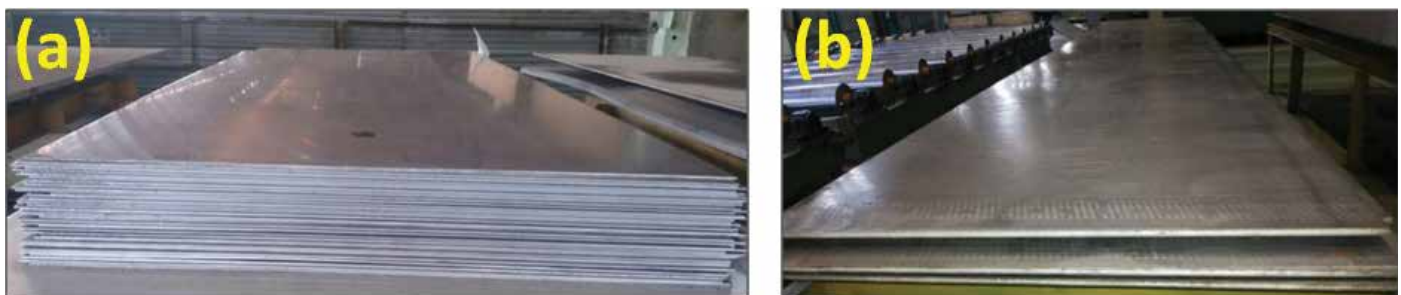
RDE40M-T7x51 sheets of thickness (a) 6 mm and plates of thickness (b) 20 mm produced at BALCO, Korba
