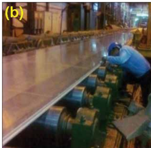
Indigenised Al-Mg alloy DMR291A in the form of (a) as-cast ingots, (b) M plate (t = 25 mm), and (c) H24 sheets (t=2 mm) produced at BALCO, Korba
