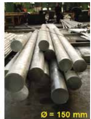
Indigenised AA6082-T651 extrusions produced at OFAJ, Nagpur
