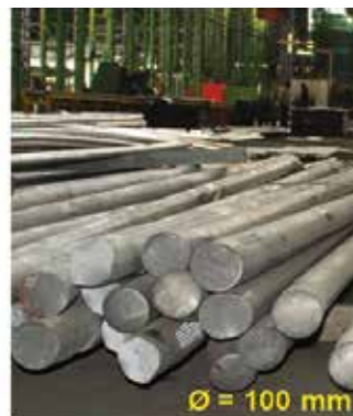
Indigenised AA6082-T651 extrusions produced at OFAJ, Nagpur
