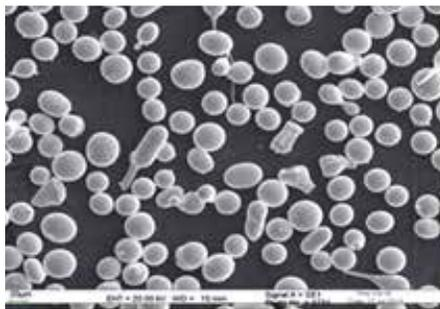
SEM images of Fe base amorphous powders of size ranging from 25 to 50  $\mu\text{m}$
