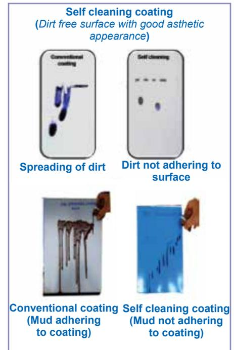
comprises hydrophobic PDMS resin and epoxy resin, which provide anticorrosive and self cleaning properties in a single coat application. The hydrophobic top surface ensures self cleaning of dirt and contaminants, while the epoxy layer underneath provides anti-corrosive properties and excellent adhesion to metallic substrates. This coating can be applied on superstructure and interior compartments of ships as well as for multifarious civilian applications.
