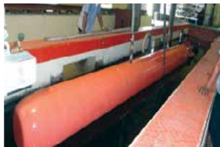
A model coated with NMRL developed drag reducing coating
