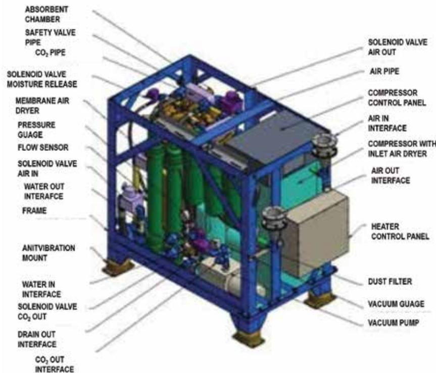
**Schematic of the CO<sub>2</sub> adsorption system with various components**
