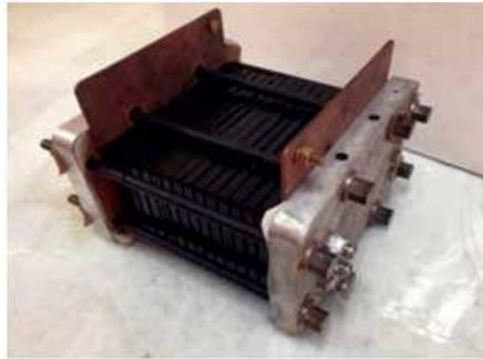
**A 100 W PEMFC stack prepared from indigenously developed nanocomposite membrane**
