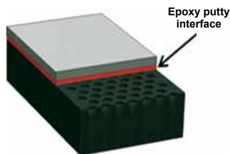
Schematic of tile-metal adhesion with epoxy putty
