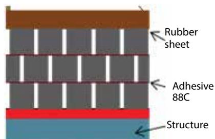
**Schematic of the application of NMR51K and NMR88C adhesives**
