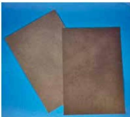
Porous conducting carbon
