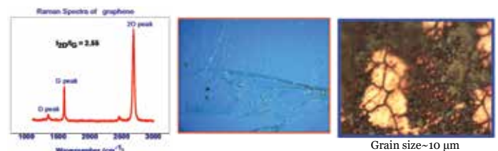
Figure 28. (a) Raman Spectra (b) FESEM and (c) Optical micrograph showing Graphene grains
