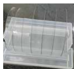
Figure 25. Diameter 4H-polytype Semi-insulating SiC Wafers and Specifications
