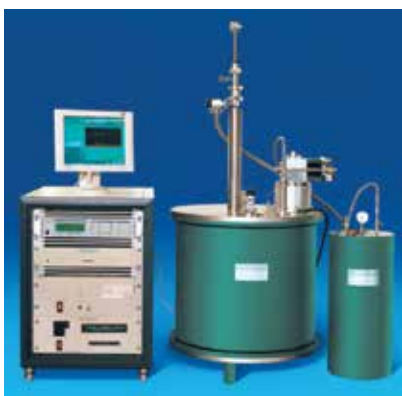
Figure 45. The Cryo-state with Electronic System for Measurement of Magneto Transport
