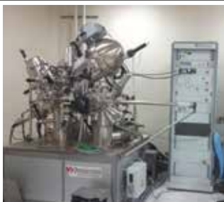
Figure 35. XPS System at SSPL
