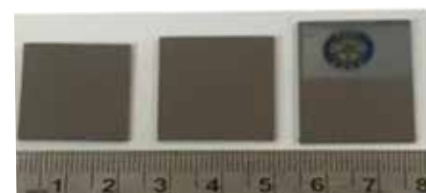
Figure 6. (a) MCT Epilayers Grown on CZT Substrates
