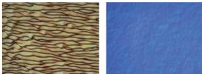
Figure 6. (b) Microscopic Surface (1350 mm X 1010 mm) of as-grown Epilayer and Polished Device Epilayer Surface
