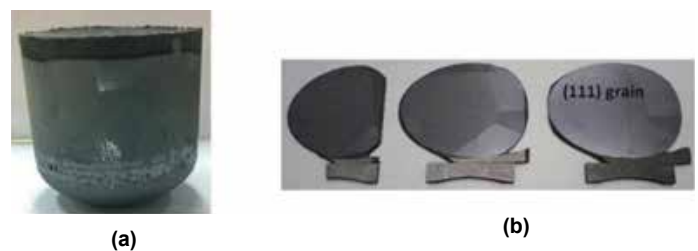
Figure 4. Technological Up-gradations, (a) Crystal Diameter Increased to 70 mm, and (b) Water Size Increased
