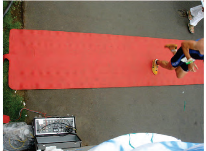
Figure 8. An RFID-based mat to sense the tags installed on the athletes passing over it.
