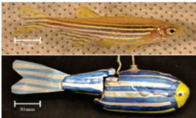
Figure 2. Comparison of the robotic-fish to a zebra fish individual.
