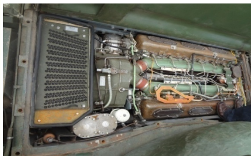
Up-rated 1000 hp Engine integrated in T-72 Tank
