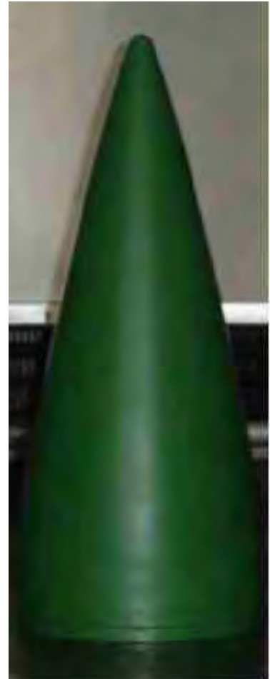
Fabricated Ceramic Radome and Joined INVAR Metal Bulkhead Ring with Glass fret technology
