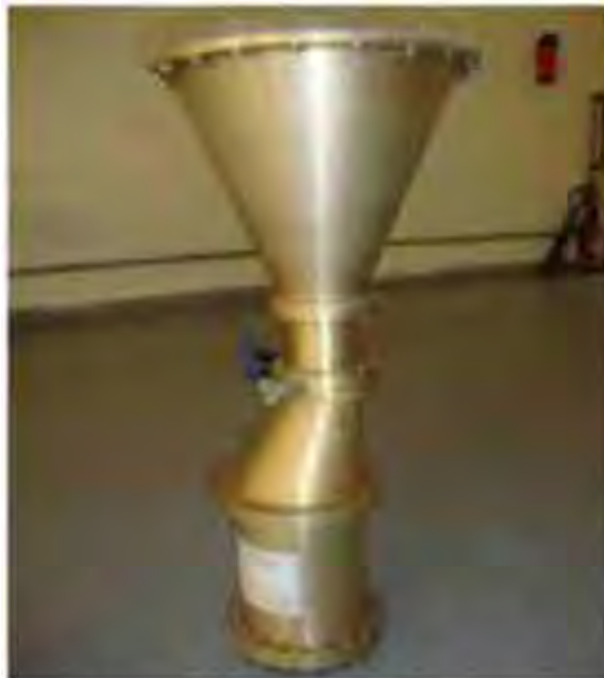
Vacuum sealed HPM Antenna
