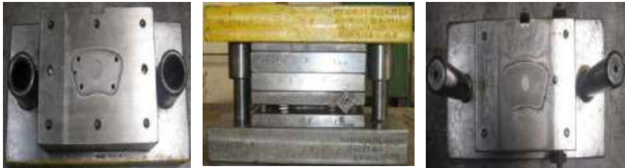
Fig 6.4: sectional and assembly view of the blanking tool
