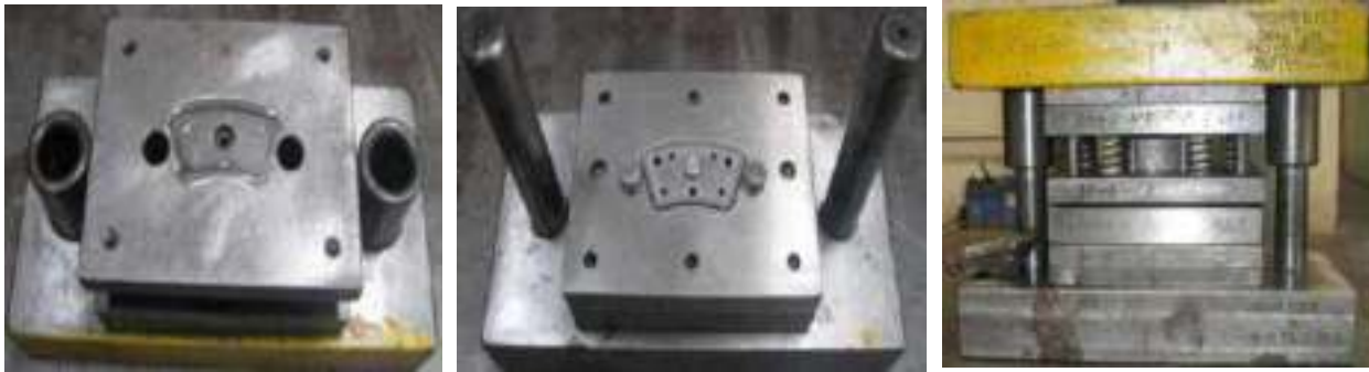
Fig 6.5: sectional and assembly view of the Forming tool
