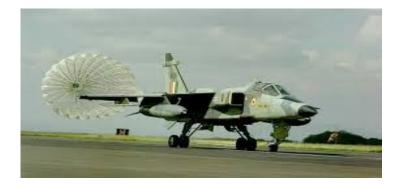
The Brake parachute system is fabricated using various textile materials and metal parts. It consists of following major components/subsystems-
