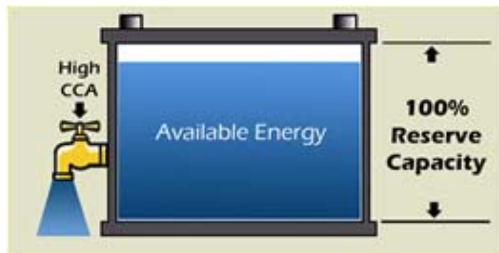
Figure 1-15 Battery with high CCA and 100% reserve capacity
