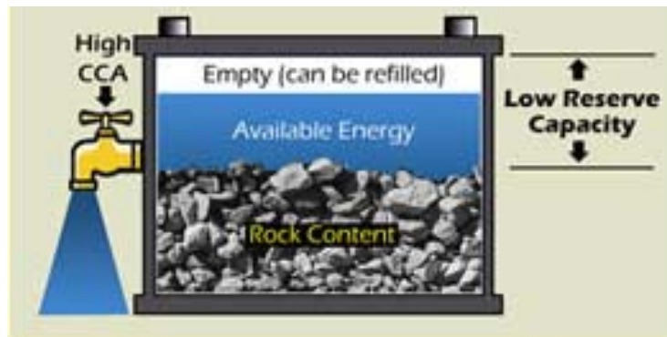
Figure 1-16 Battery with high CCA but low reserve capacity
