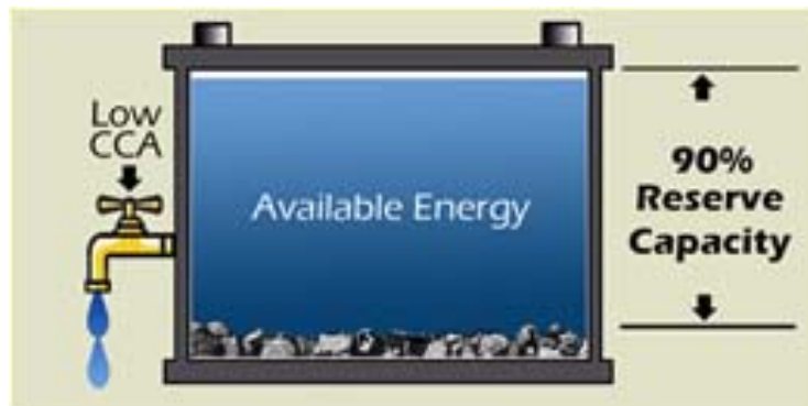
Figure 1-17 Battery with low CCA but high reserve capacity
