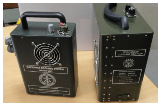
AMCCS chiller Units (backpack and twin crew configuration)
