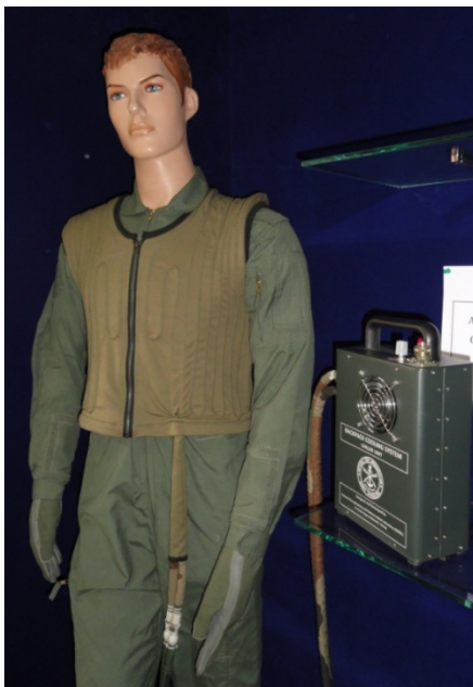
AMCCS with LCG and Chiller Unit
