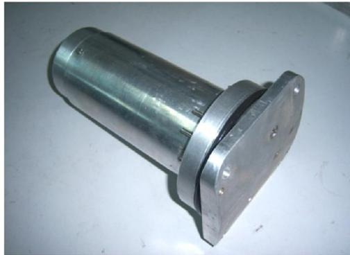
Exploder is a critical subsystem of Naval warhead, which ensures safety of the warhead in transportation, handling, storage and operations. Exploder prevents inadvertent arming and detonation of warhead by removing all safety interlocks and initiating explosive train only when intended.
