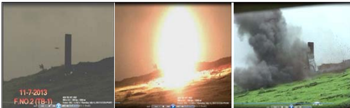
Figure 5. Thermobaric ammunition of 105mm IFG breaching a brick wall of 400mm thickness.
