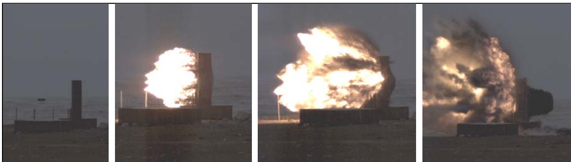
Figure 3. 120mm thermobaric ammunition of MBT Arjun defeating RCC target structure of 500mm thickness.
