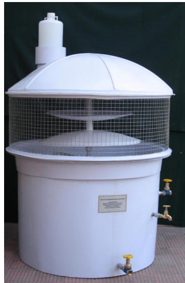
Dearsenification Unit (Capacity 200 L/Hr)
