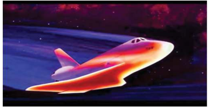
Figure 6. NASA space shuttle orbiter re-entering Earth with a 40° angle of attack.
