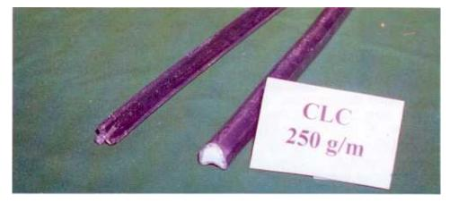
250 g/m flexible linear shaped charge
