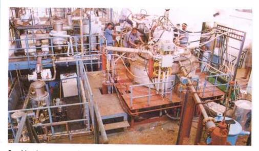
Combined process equipment for Ti sponge production in 4000 kg batches
