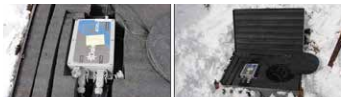
Figure 14: AE Node Installed in Avalanche Formation zone.
