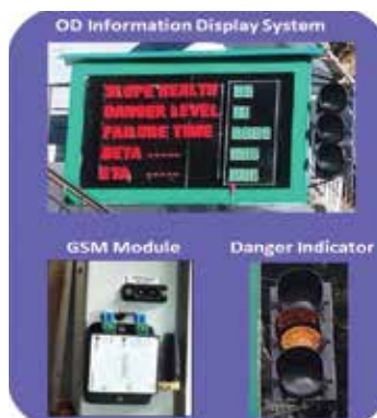
Figure 18: Avalanche Information Dissemination through Outdoor Display Signboard (top), GSM Message Alerts (bottom left side) and Traffic signal Danger Level Indicator (bottom right).
