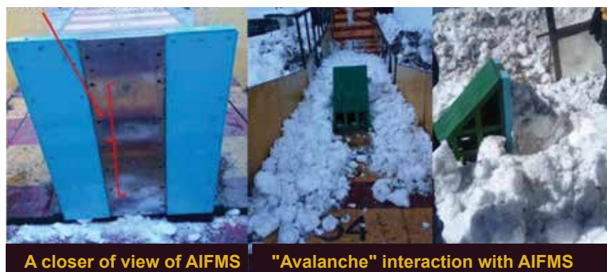
Figure 25: AIFMS system installed in avalanche chute and interaction results
