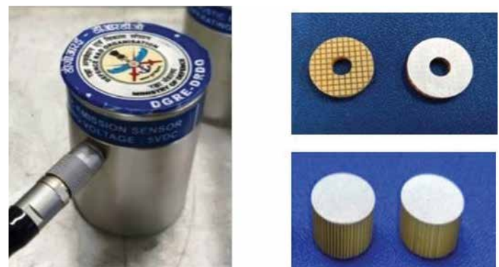
Figure 12: Indigenously Developed AE Sensing Unit (left) Based on 1-3 piezo Composite Material (right).
