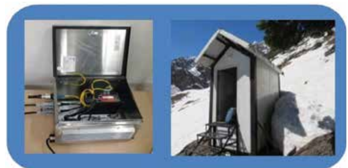
Figure 15: AE Hub with OFC Data Interface, Housed Inside Shelter Installed Near Avalanche Formation Zone.
