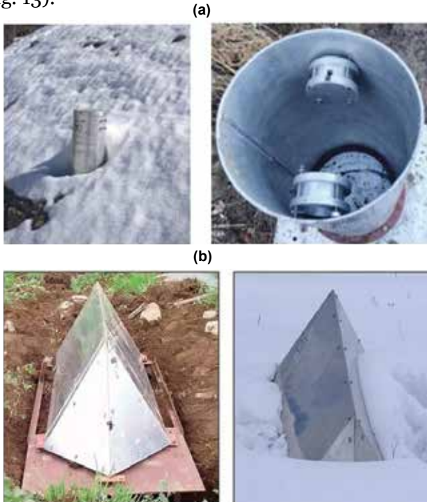
Figure 13: AE Arrestors installed in Avalanche Slope, (a) Static (OD-AR) types of AE Arrestor (left) and Sensor Housing (right), (d) Dynamic (WS-AR) types of AE arrestor.
