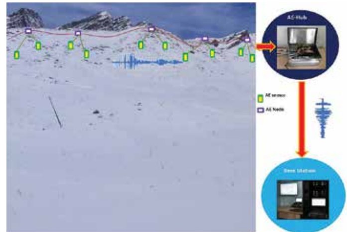
Figure 11: Site-specific AE Sensor Networking in Avalanche Formation Zone
