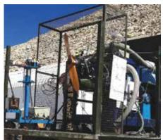
Turbocharger EFI Engine on mobile test platform at Chang La (17,500 ft)
