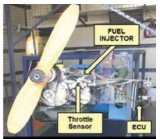
Rotary engine with EFI system on test bed
