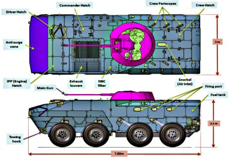
Wheeled Armoured Vehicle and its Structural Diagram (below)
