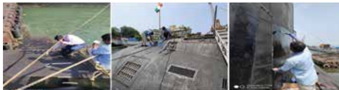
Field trials of black and white protective paint onboard Submarine
