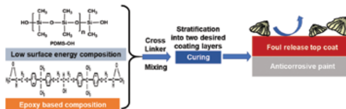
Self-stratification mechanism of the foul release coating
