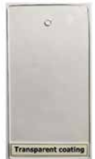
Perspex acrylic sheet coated with transparent coating
