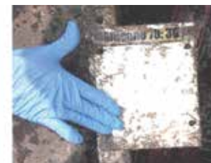
Foul release coating after 90 days of immersion
