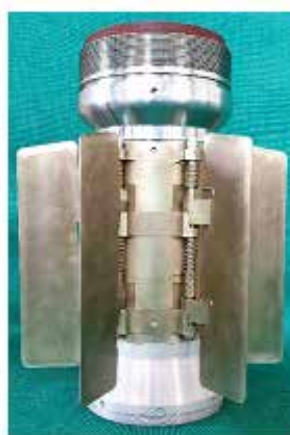
Stabilizers for Pinaka Mk-I, Mk-II and Guided Pinaka Rockets
