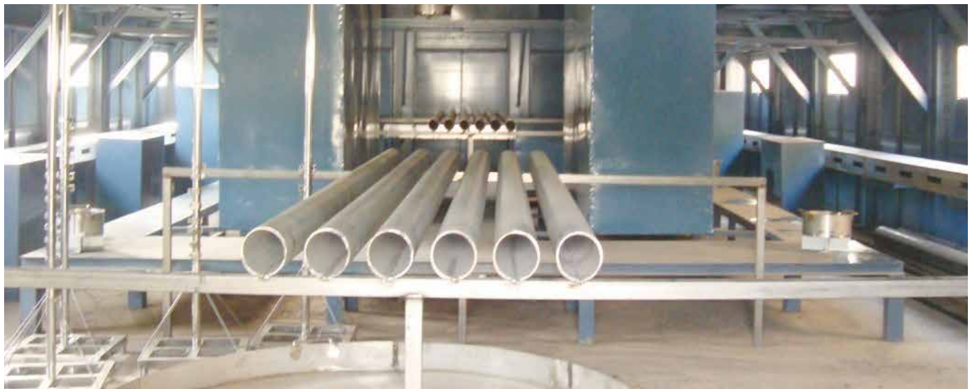
Inside view of the 1000 m 3 fire simulation facility with ship engine mockups
