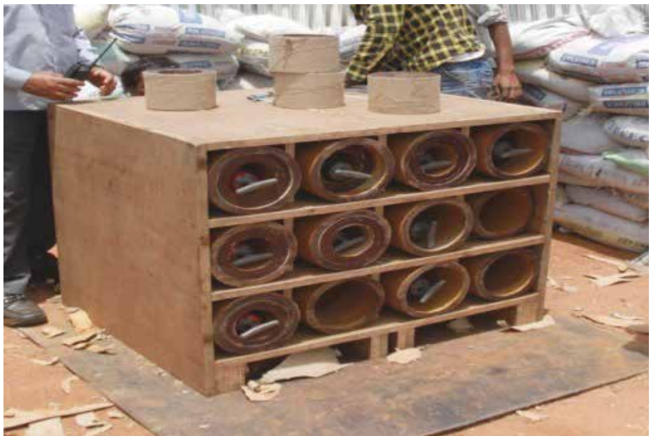
Modified packaging of HEER shell 155 mm
