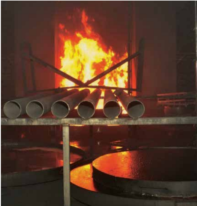
2.5 m diameter pool fire under the bilge plate & engine mock-ups
