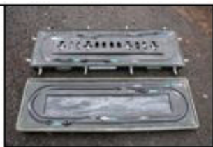
Canopy Severance System Package in open condition
