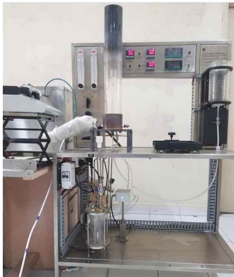
Semi-automatic standard-cup-burner setup
