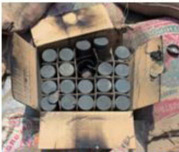
No Propagation to adjacent packages (Single Package Test)
