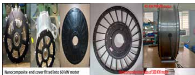
Nano-composite-based Structures for Torpedo Propulsion Motor
