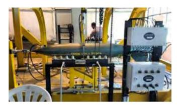
strain gauges and LVDTs, respectively. Load cells, strain gauges and LVDTs are connected to a 80-Channel Data Acquisition System (DAQ). Parameters are monitored and recorded using the DAQ. The maximum size of the bomb which can be load tested is 600 mm x 4000 mm.
