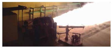
The 33T class (Thrust) solid rocket motor is one of the largest rocket motors with HD1.1 class of propellant in a composite casing being processed in India. The static testing of the motor involved data acquisition of 30 channels for temperature, 36 channels for strain, 2 channels
