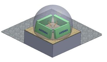
to detect targets in excess of 400 Km in range. The radar is required to classify targets automatically and have advanced ECCM features. The Radar will be capable of resolving target in four dimensions (4D) namely Range, Azimuth, Height and Doppler Velocity. The Radar will have the capability to interface with IFF system and correlate with the target data.
