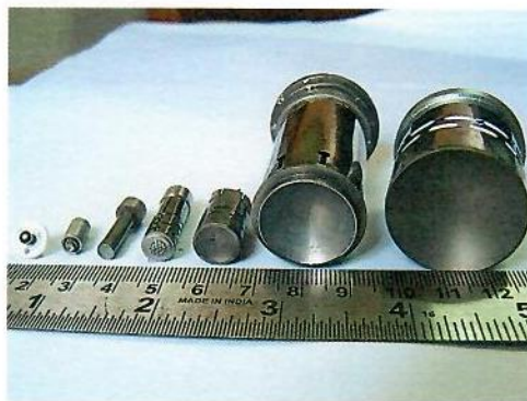
Figure: Photo of dispenser cathodes developed at MTRDC. Cathode diameter ranging from 1.4 mm to 30 mm, for various vacuum microwave devices.
