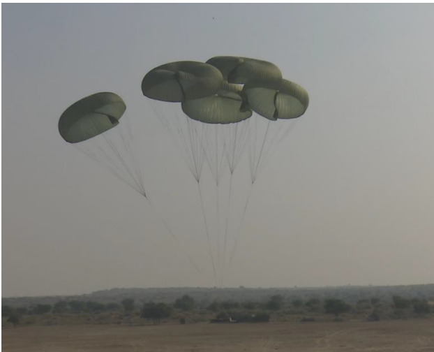
Fig 3: Fully deployed HDS during descent
