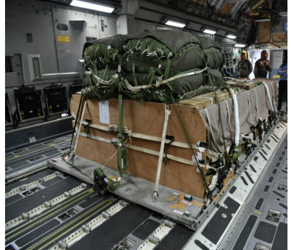
Fig 2: HDS secured inside aircraft
