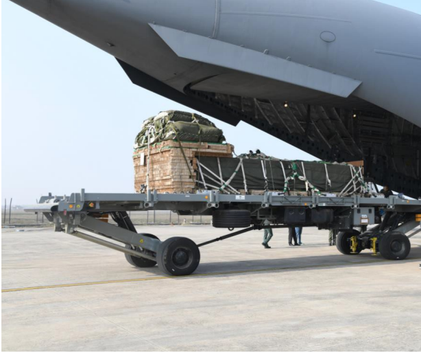
Fig 1: HDS during Aircraft Loading
