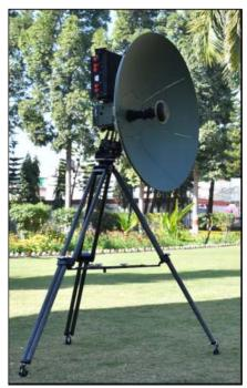
assembly and alignment & pointing mechanism with light weight tripod. It can support ranges up to 60 kms path lengths in Troposcatter mode and 100 km path length in Line of sight (LoS) mode. CTCS link prediction software with integrated GIS data is included in the system for link planning and link feasibility in offline mode.
