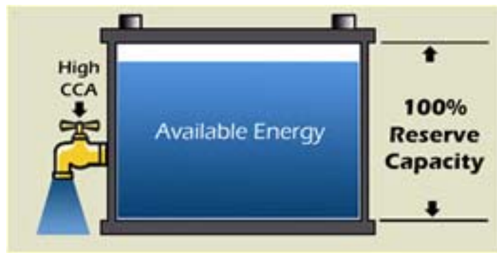
Figure 1-15 Battery with high CCA and 100% reserve capacity
