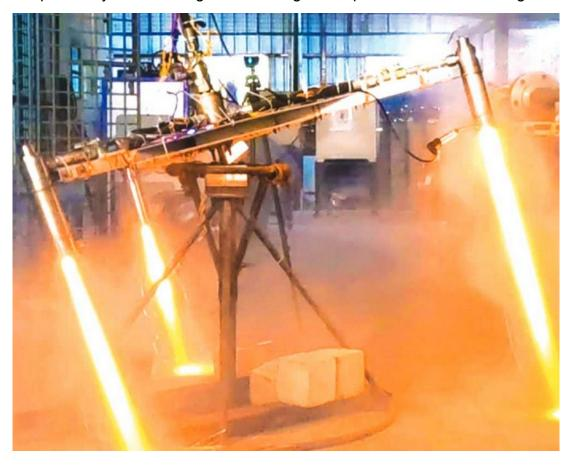
Currently, VTOL systems are complex and require high maintenance. Therefore, the researchers conceived the concept of a hybrid rocket thruster-powered platform as part of a system development study to develop an effective propulsion unit for achieving VTOL in aircraft and UAVs. According to PA Ramakrishna, professor at the Department of Aerospace Engineering, IIT Madras, VTOL enables an aircraft to take off and land vertically, eliminating the need for infrastructure like long runways.
