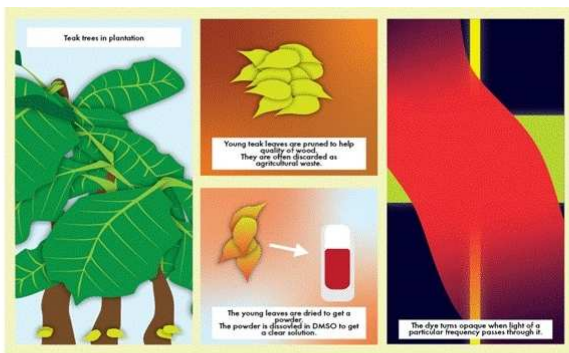
Fig 1: The process through which Teak Leaf extract is prepared to study the nonlinear optical properties.
