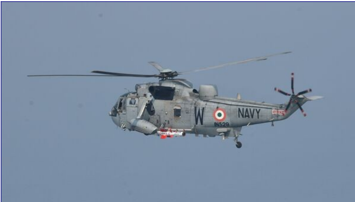
An Indian Navy Sea King Mk 42B helicopter prepares to launch a Naval Anti-Ship Missile-Short Range during trials off the coast in eastern India on 25 February 2025. (DRDO) (2066876)
