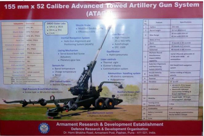
The ATAGS is a 155 mm/52 calibre gun with a theoretical firing range of 40 km. The gun currently weighs about 18 tonnes, while the ideal weight for the army would be 14-15 tonnes. The Indian Army has begun finalising the preliminary specifications qualitative requirements (PSQR) which should be completed by July 2019, reported The Times of India. In the earlier trials which were conducted in December 2018, the gun had fired on targets distant of 47.2 km.
