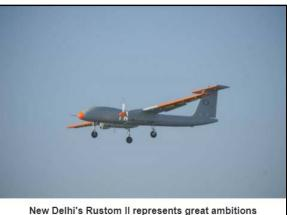
TAPAS 201 features lofty specifications, such as an operating altitude of 30,000ft, a service ceiling 32,000ft and the ability to take off from runways as high as 11,000ft. The 2t-class MALE UAV will be able to carry a payload of 350kg (770lb) and undertake intelligence, surveillance and reconnaissance missions for the Indian army, air force and navy.
