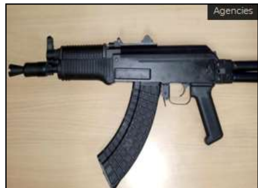
TriCa has a special muzzle booster which helps in hiding the flash and mitigating the sound when fired
