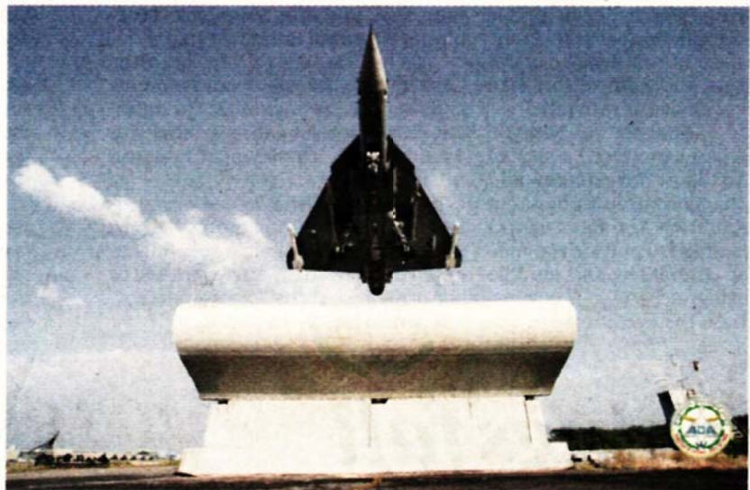
The Tejas prototype took off from the Navy's SBTF, but exactly as it would have from an aircraft carrier. Restraining gear locked the fighter's wheels as the engine revved up to maximum power
