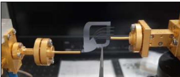
Experimentation with the multiplexer, showing connection to external systems. The multiplexer does not have any form of supporting substrate. Credit: Osaka University
