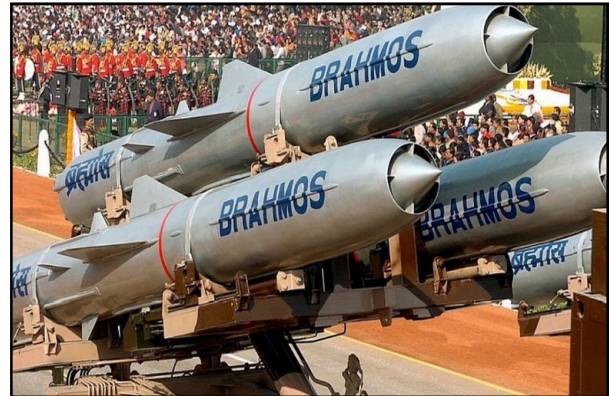
BrahMos is an Indo-Russian ramjet-powered supersonic cruise missile based on the Russian P-800 Oniks supersonic anti-ship cruise missile. Credit: Twitter.
