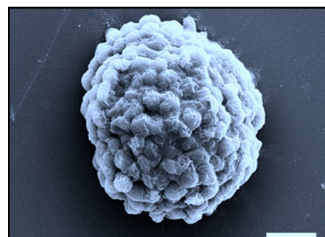
Electron microscopy image of a densely packed droplet of hydrogen-producing algal cells. Scale bar, 10 micrometres. Credit: Prof Xin Huang, Harbin Institute of Technology
