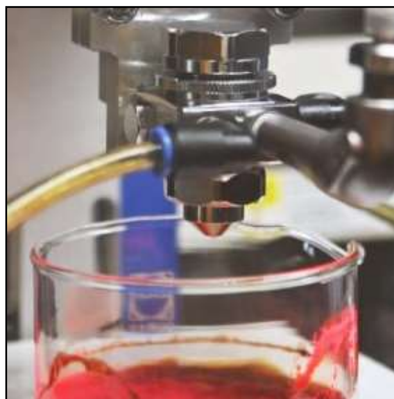
Professor Hao-Wu Lin of the Department of Materials Science and Engineering at National Tsing Hua University in Taiwan has developed a spray-synthesis method for preparing perovskite quantum dots with a uniform protective organic layer. Credit: National Tsing Hua University
